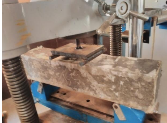
Fig 3.5 Flexural test on Beams
