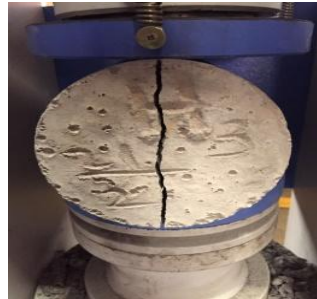
Fig: 3.3 Split tensile test on cylinders
